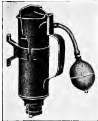
Fig. 6. The Wisconsin milk sediment test.
